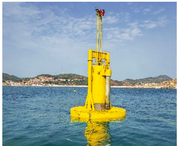
Shandong University wave energy device in sea trial
