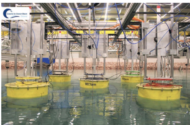
The experimental setup of the five-WEC array the Coastal and Ocean Basin Ostend: overview and detail.
