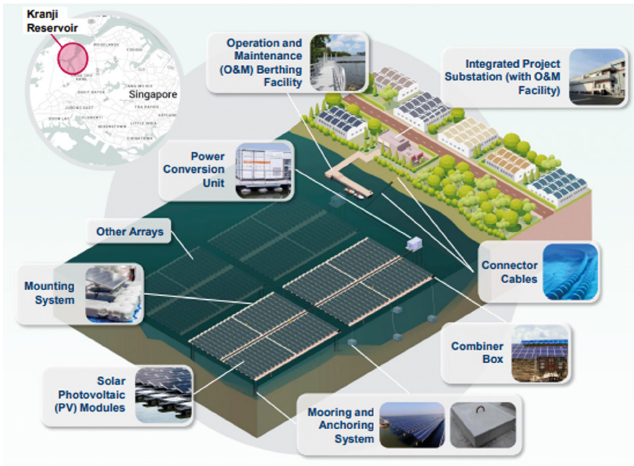
Figure 9: Floating Solar system planned in Kranji Reservoir
