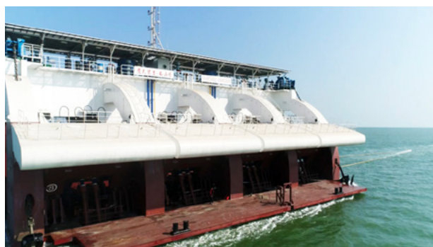
500 kW “Zhoushan” and 500 k “Changshan” wave energy platforms
