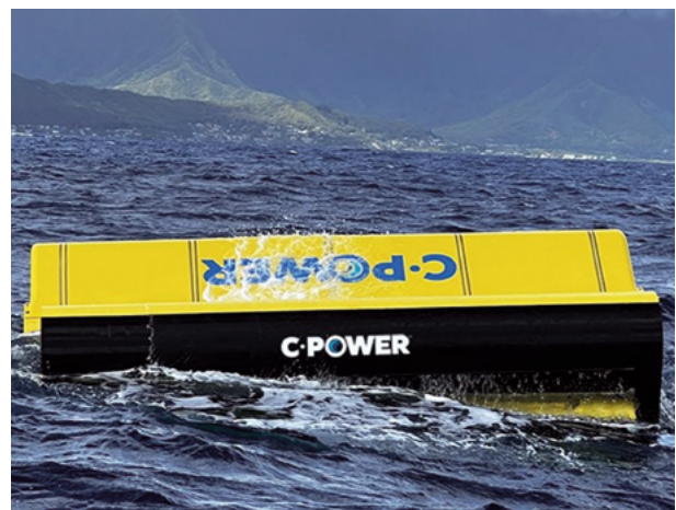
Developer C-Power conducted a second-phase deployment of the SeaRAY AOPS at the Wave Energy Test Site in Hawaii (1. In-harbor operational testing; 2. Open water demonstration). © C-Power
