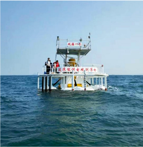
Guanhai I wave energy buoy in sea trial
