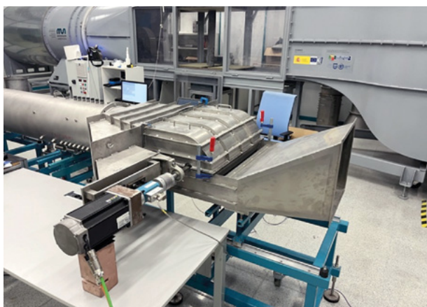
OWC solution been tested at a 1:85 scale at the facilities of Mondragon Unibertsitatea. © Arrecife Energy Systems
