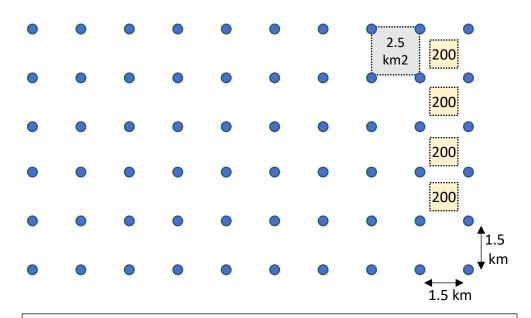
125 km2 wind farm of 750 MW + 750 MW
