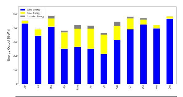
NL Simulation based on OOE-OSI1 Model 2020 data from LaRC PowerProject API service 1000 MW of offshore export, wind, & solar
