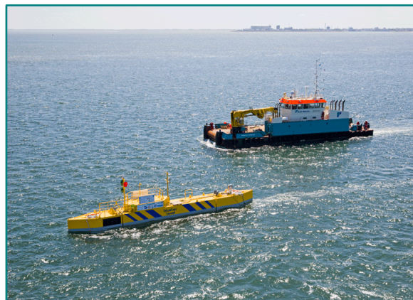
BlueTEC floating tidal power
